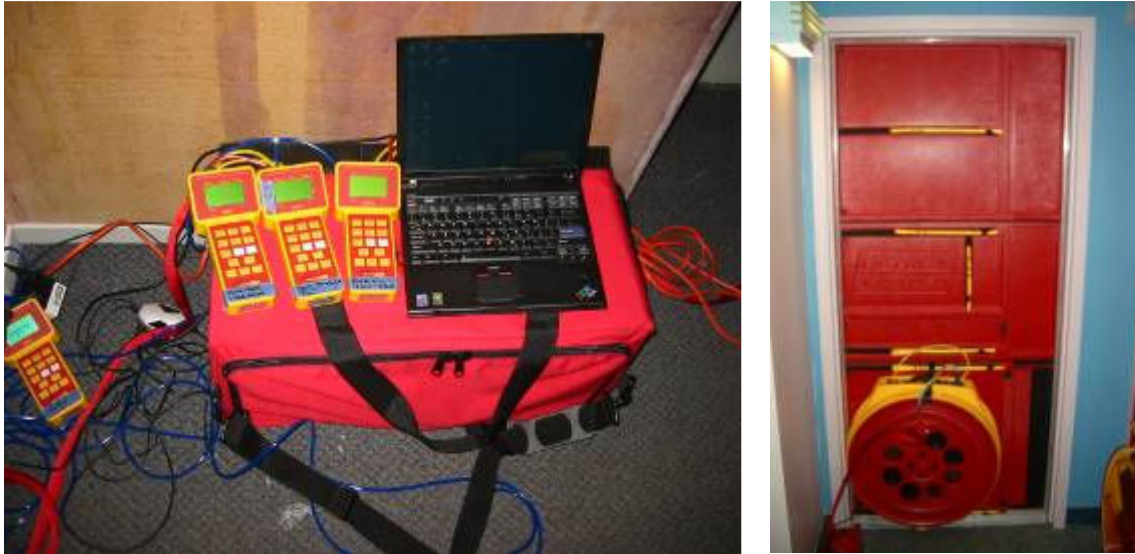
Figure 1-2: Control Equipment and Door-Fan Installed in Hallway Doorway.
