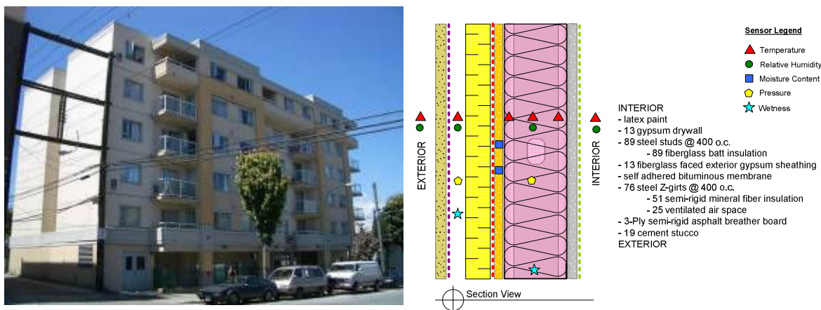
Figure 1-6: Building 3 – Overview and Wall Assembly Details
