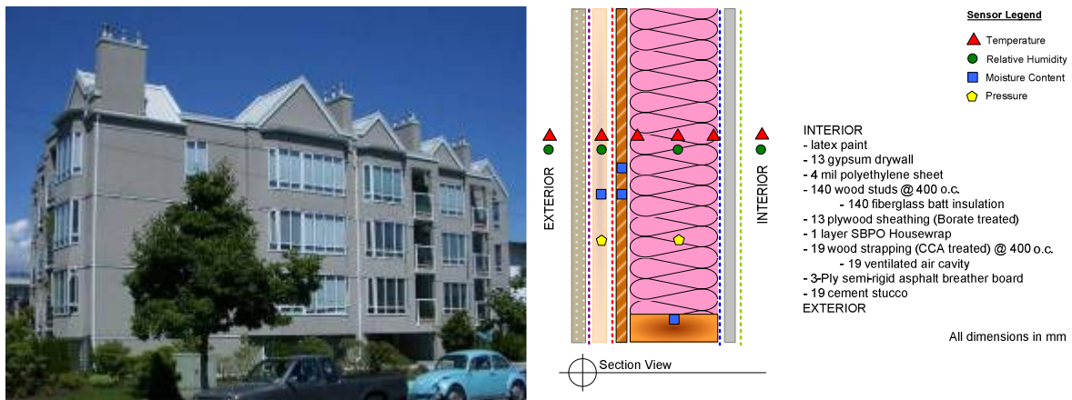
Figure 1-3: Building 2 – Overview and Wall Assembly Details.
