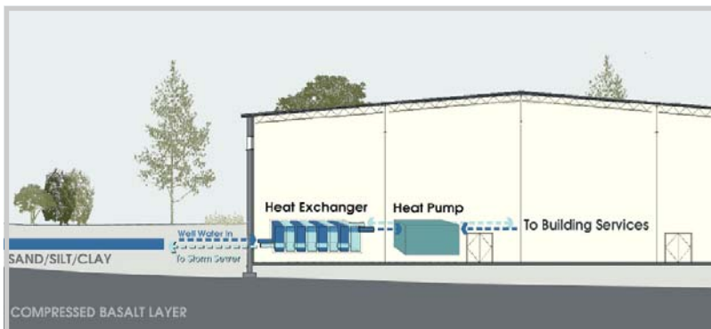
Ground water is captured and used to operate ground source heat pump (and also to irrigate ball fields.) Graphic courtesy of Boora Architects
