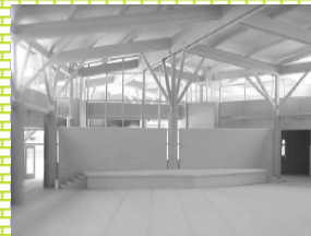
Daylight modeling helps designers see the patterns and penetrations of light during different times of the day and year.
